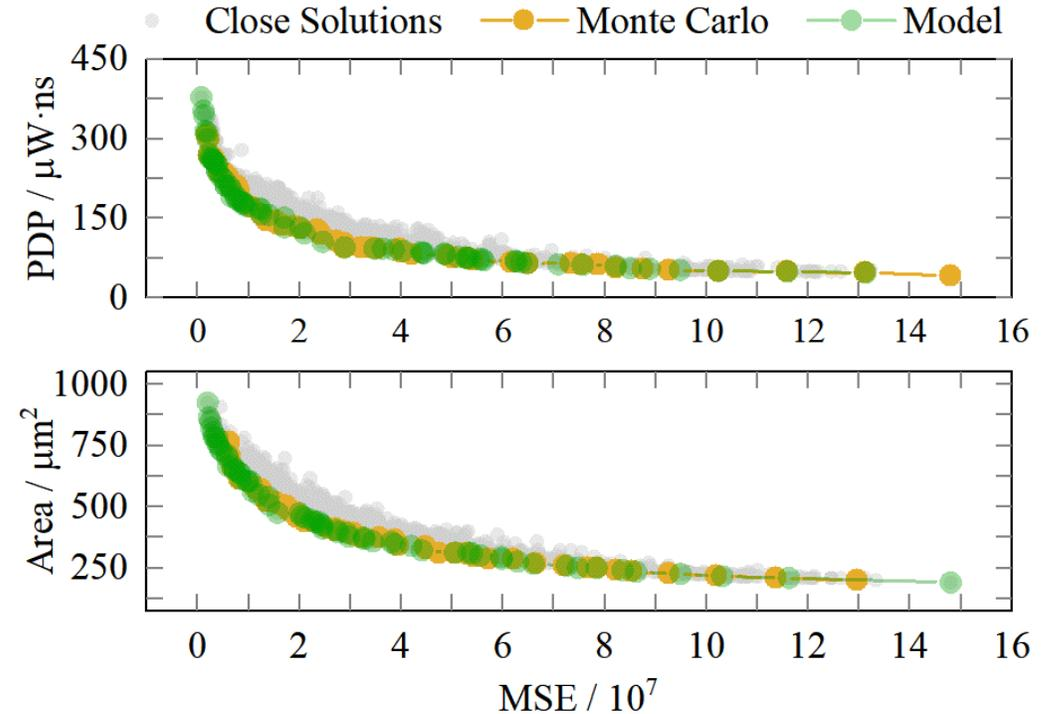
Fig.4: The Pareto-optimal values using the proposed model and Monte Carlo method.
