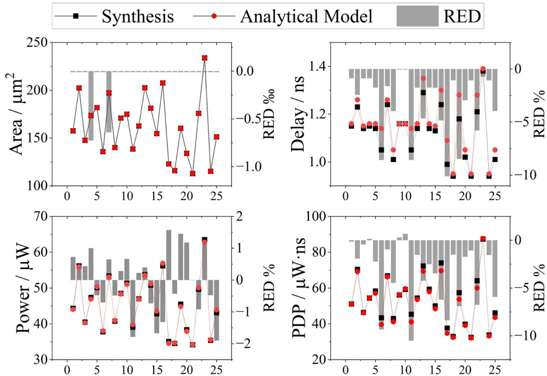
Fig.2: Hardware evaluation using 25 representative multipliers for area, power consumption and PDP.
