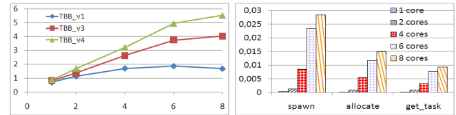
(a) Speedups. The x-axis represents the number of cores (b) Ratio for library functions in TBB_v3 and TBB_v4
